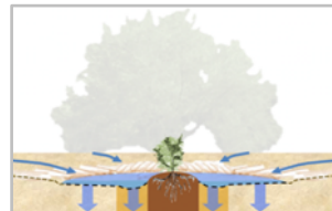
Place tree on slightly raised planting area if inside a water harvesting basin to protect trunk from frequent inundation
